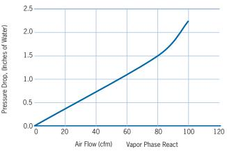
Pressure drop through a VENTSORB unit is a function of the process air flow as shown in the graph. A VENTSORB canister can handle up to 100 cfm at a pressure drop of less than 2.5 inches of water column. If higher flows or lower pressure drop is needed, multiple canisters may be installed in parallel operation. The maximum canister pressure should not exceed 4 psig.
