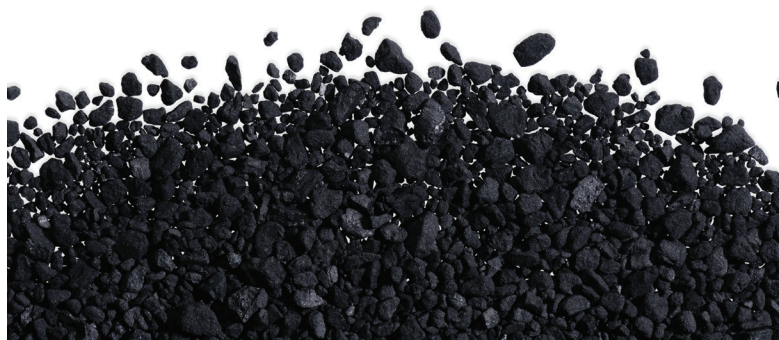
FIGURE 1. Activated carbon is used in treatment processes when manufacturing a wide variety of industrial products, as well as in environmental treatment for water, air and more
